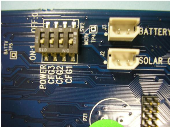
The OFF position for CFG2 enables the external power regulator circuit inside the unit.
